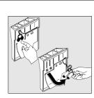
You can thus clean it using running water and a brush or a twisted cloth. Check that the siphons at the back of the detergents dispenser are not blocked.
